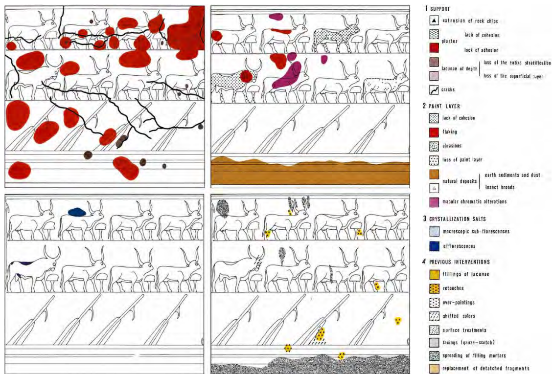
>> Figure_4.2.02. Inspection of the condition of the side chamber [G] of the wall [G2].
